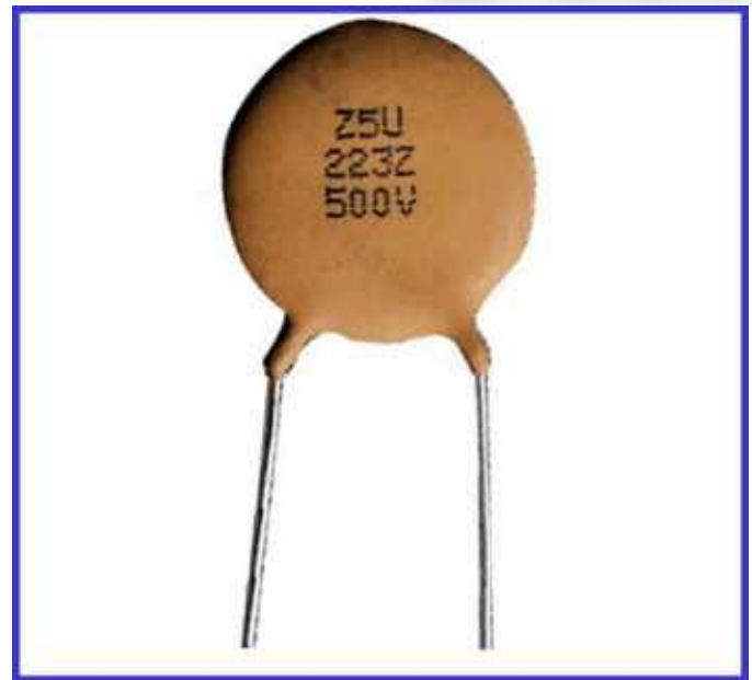
Figure 2 - A class 2 disc ceramic capacitor 0.022 µF 500V Z5U
