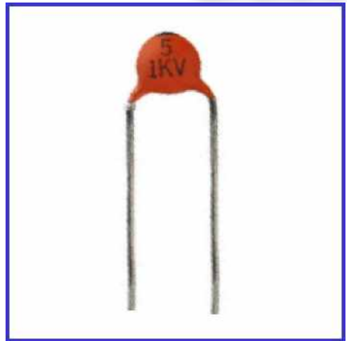
Figure 1 - A class 1 disc ceramic capacitor 5 pF 1KV C0G (NPO)
