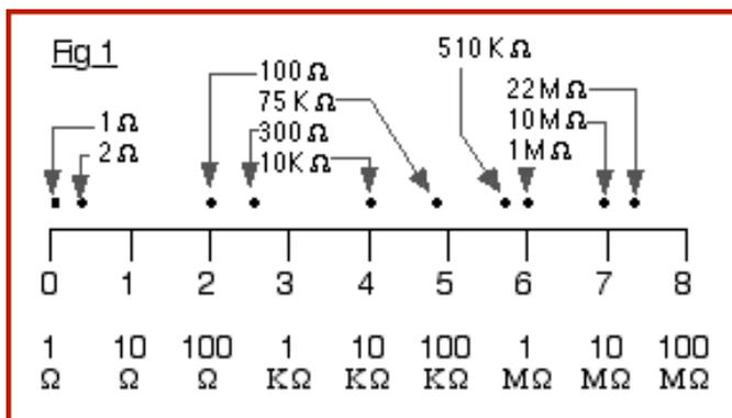
Notice in the table that orders of ten each take up the same amount of room on the bottom scale. The same axis space is given to values between 1Ω and 10Ω as between 100KΩ and 1MΩ. Thus the space between
