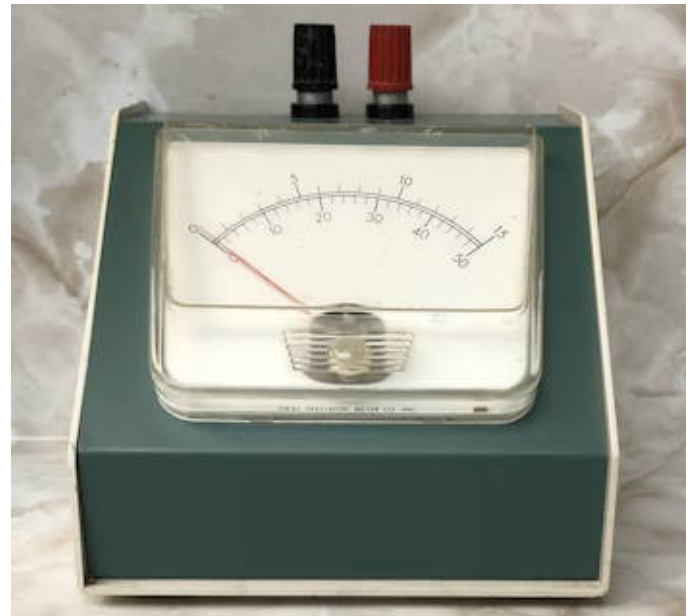
Figure 1: Heath EUW-18 Lab Meter, 0–1 mA, 50Ω meter movement (shown less shunts).
