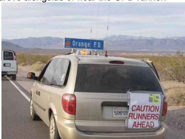
Fig 4 – The OPD Follow Vehicle with three ham antennas. Two dual-band 144/440 mag-mounts for voice and 2M antenna for APRS Beacon
