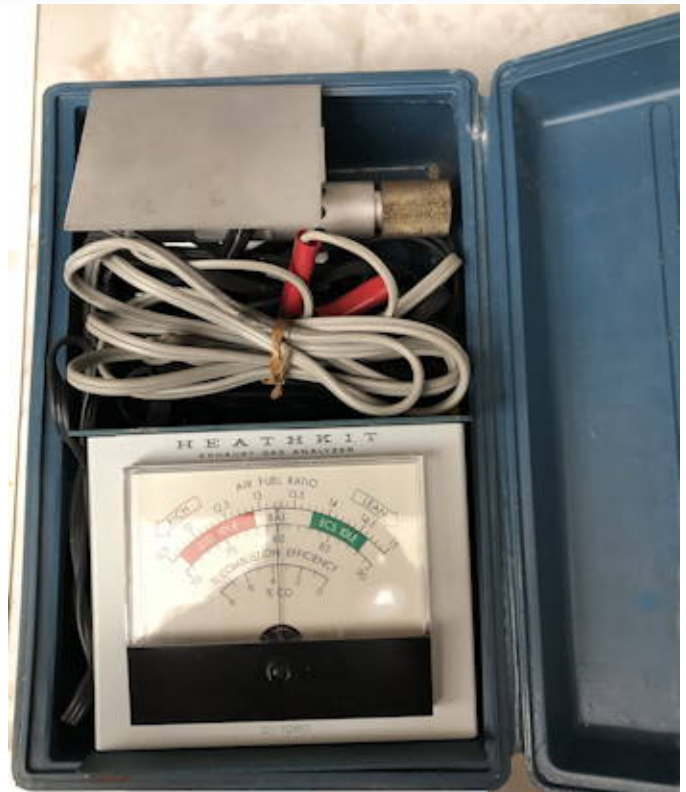
Figure 1: Author's Heathkit CI-1080 Exhaust Gas Analyzer purchased mail order in August 1974. (Apologies for the reflection on the meter face.)
