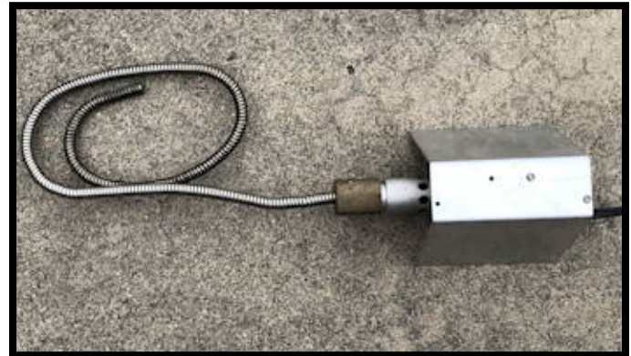
Figure 3: Probe assembly, consisting of Sensor, Sensor cover, Probe Body, Knurled Collar, & Probe Stand. Also shown attached is the flexible tube.
