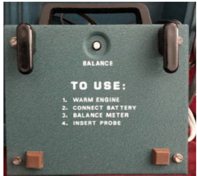
Figure 2: Rear cabinet view, showing balance control, hooked feet and simple instructions.
