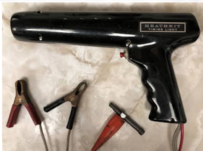
Figure 1: The Heathkit CI-1020 Timing Light showing the battery clip leads and red clip with metal spring adapter that mates between the #1 spark plug terminal and its spark plug wire, or the #1 spark plug wire and the distributor.
