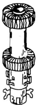
Figure 8: Part #52-101 bandpass transformer showing the two toroids mounted on a coil form. Image is of the factory supplied part from the Heathkit SB-620 manual.
