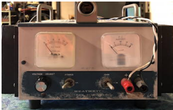
Figure 10: The author's IP-2715 as it was when it arrived to the workbench. Dirt, grime and the cigarette lighter receptacle have since been removed, and the unit is working electrically.
