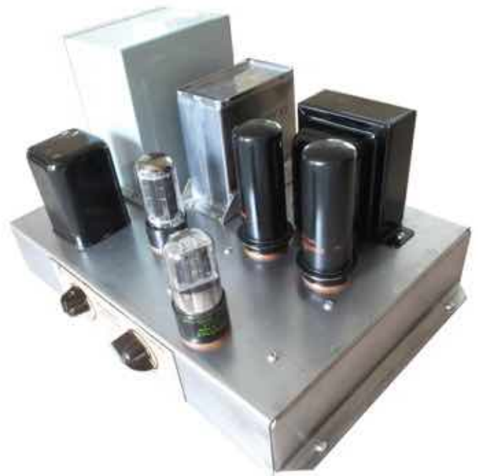
Figure 1: Heathkit A-1 High Fidelity Amplifier. Photo courtesy of Keith Greenhalgh.
