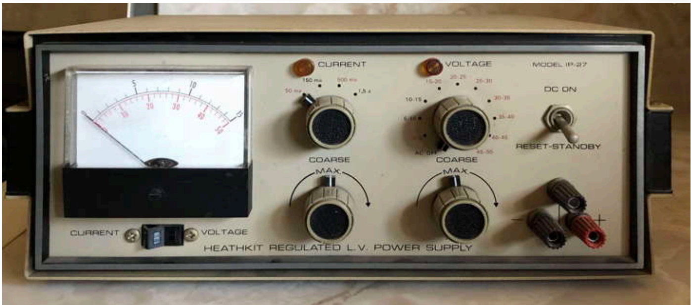
Figure 5: Front View of The Heathkit IP-27 Regulated LV Power Supply
