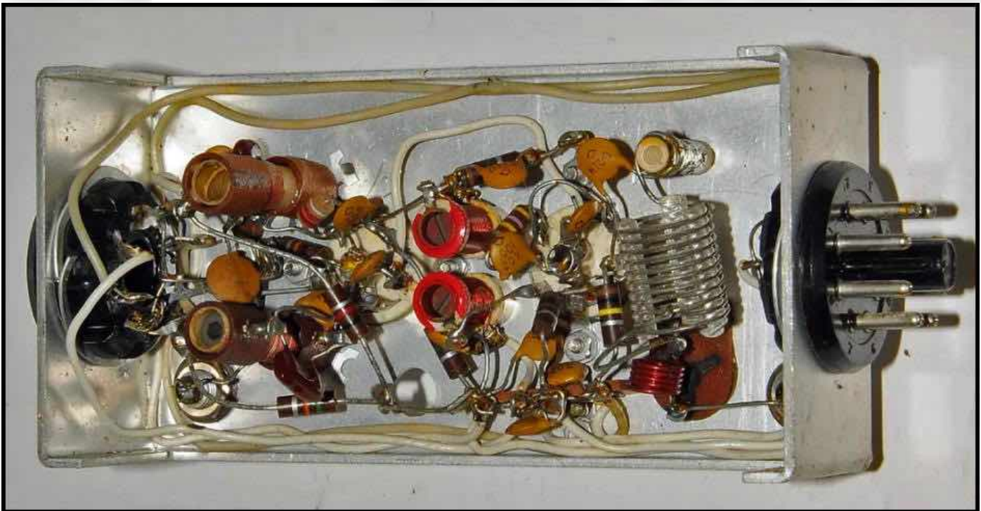
Figure 6: Inside view of the SBA-300-3 Six-Meter Converter (WA7ZZE - credit)
