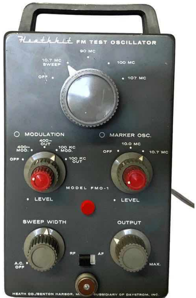
Figure 1: Heathkit FMO-1 FM Test Oscillator
