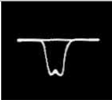
Fig. 3: 10.7 MC IF alignment scope pattern.
