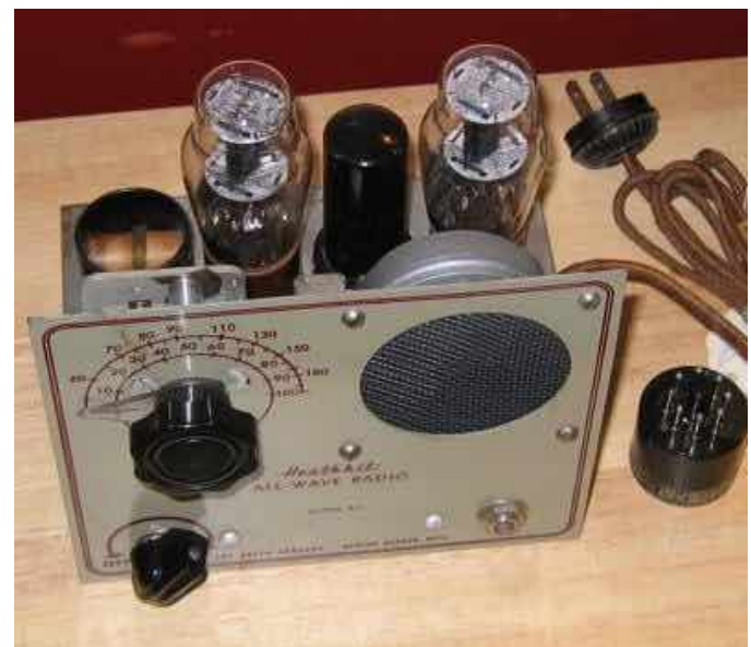
Figure 12: Photo of a K-2 from the Antique Wireless Association Museum. Note model number on front panel (lower center) and the two 1626 glass tubes that replace the 12C8 and one of the 12A6 tubes used in the K-1 Photo posted by Jim - N2EY on QRZ.
