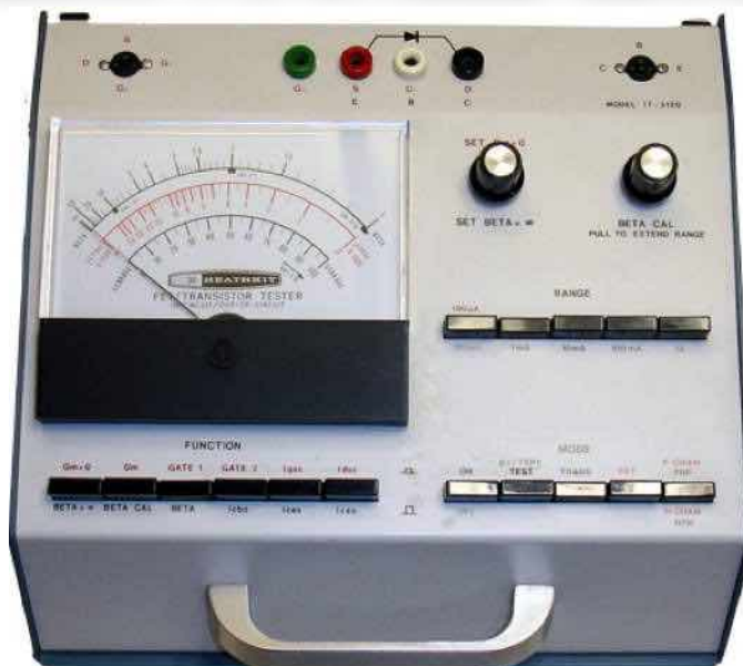
Figure 1: Restyled Heathkit IT-3120 FET / Transistor Tester
