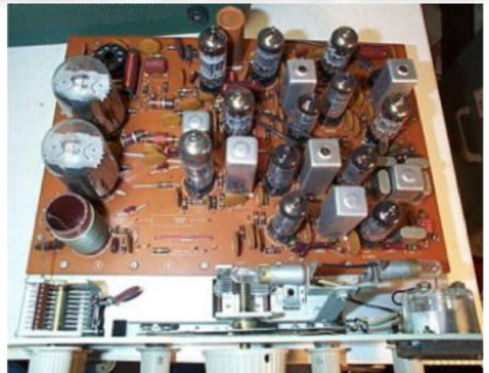
Figure 2: Top view of the HW-22 out of its cabinet. Final tubes are to the left behind vertically mounted pi-network coil. In the back left is the octal socket for the optional crystal calibrator.
