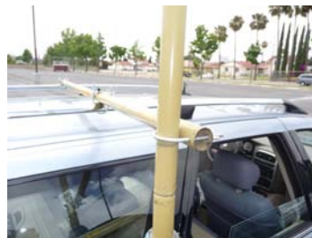
Figure 5 – Mast-brace attaches to roof-rack
