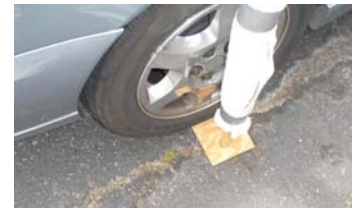
Figure 6 – The car tire secures the support base and prevents mast from slipping.
