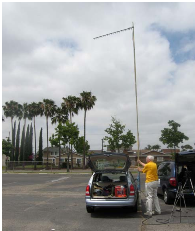
Figure 4 – Bruce KC6DLA adjusts direction for the Field set-up of the 1.2 GHz Loop-Yagi
