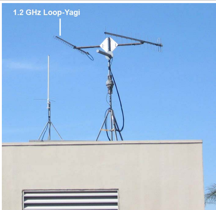
Figure 3 – 1.2 GHz Loop-Yagi on roof of OPD
