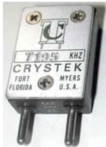
FT243 Style Crystal used by most popular Novice rigs in the late '50's and early 60's. Figure 1
