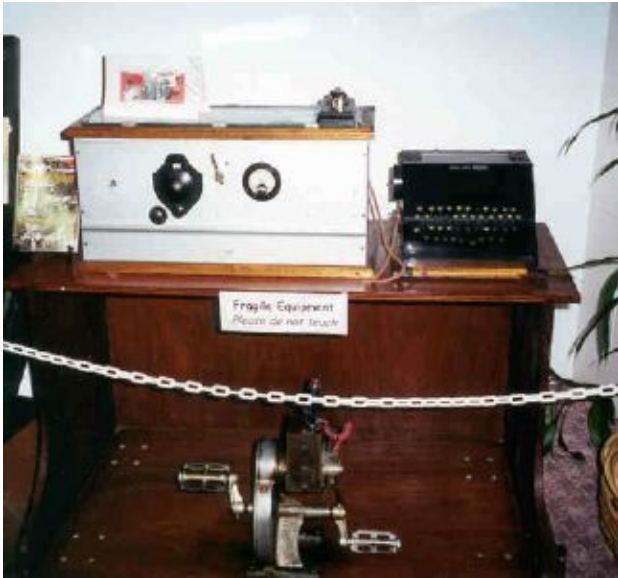
The first pedal powered transmitter and receiver with code machine
