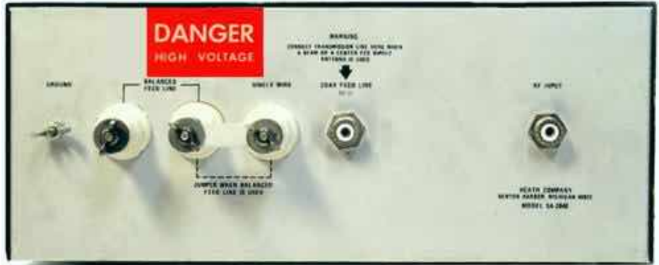
Figure 3: Heathkit SA-2040 Rear Panel. Outputs are on the left. Input is on the right.
