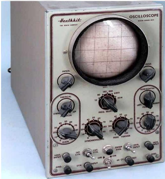
**Figure 7:** The Heathkit O-2 Oscilloscope. Photo courtesy of Chuck Penson - WA7ZZE
