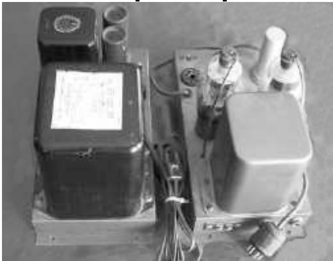
Fig. 2: Heathkit W-1. Power Supply is on the left, Amplifier Chassis is on the right.
