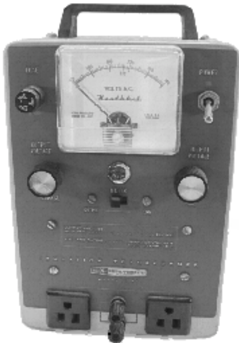
Later Heathkit IP-22 Isolation transformer
