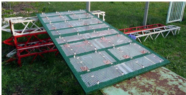
Fig 5 – Large 6-loop panel array construction by HA5IW (Courtesy of Paul G8GML)
