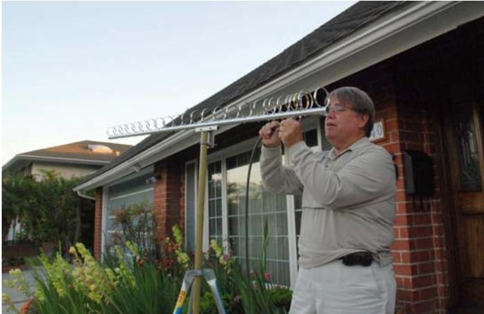
**Figure 10 – COAR Member KB6CJZ measures SWR on 1.2 GHz “Elephant Gun” Loop-Yagi**
