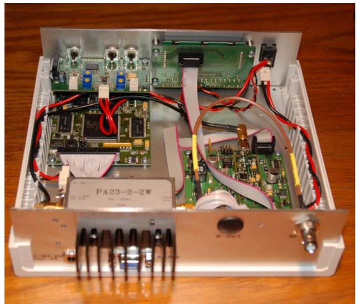
**Figure 2 – View of KomplettSender transmitter from rear with top cover removed**
