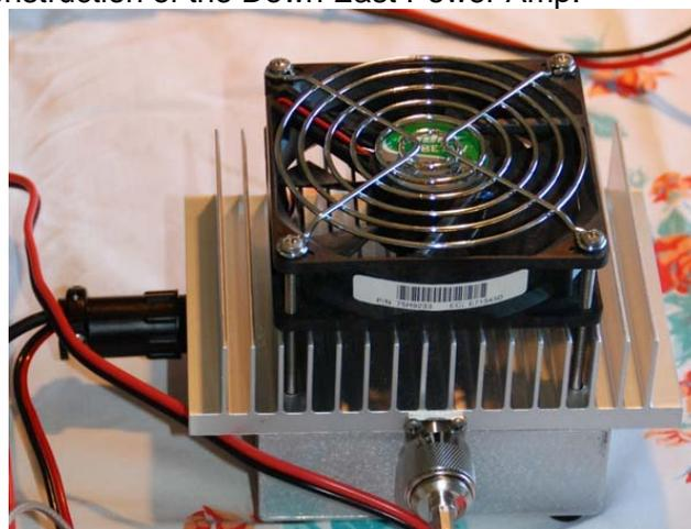
**Figure 6 – Construction of Down East Model 2330PA Power Amplifier**
