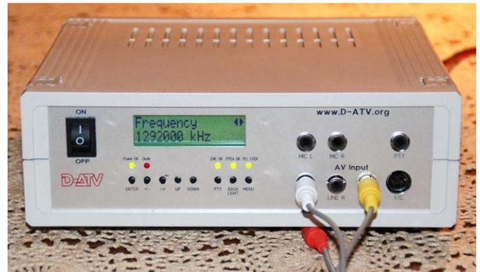
**Figure 3 – Front panel of KomplettSender with LCD Display and Menu Controls**
