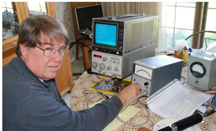
**Figure 7 – Robbie KB6CJZ is shown with HP Model 432A Power Meter and HP Model 8559A Spectrum Analyzer 0.01-to-21 GHz plug-in**
