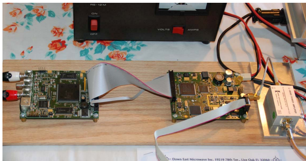
Figure 2 – Breadboard of MPEG-2 Board and MiniMod Exciter Board and Kuhne 1 st -Stage PA
