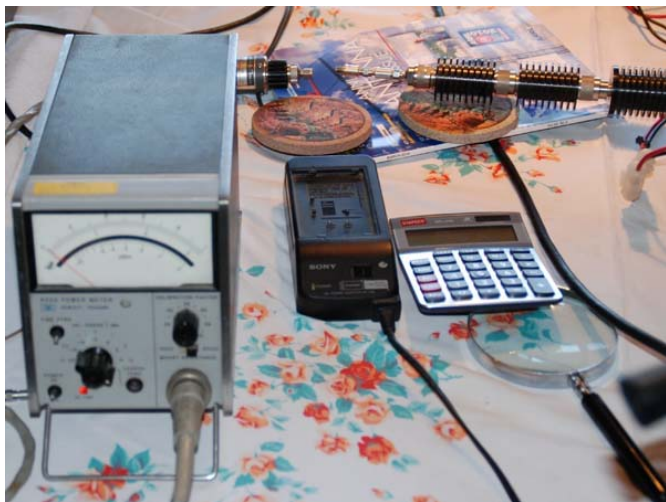
Figure 5 – HP Model 432A Power Meter Note attenuator-stack at the top of the photo
