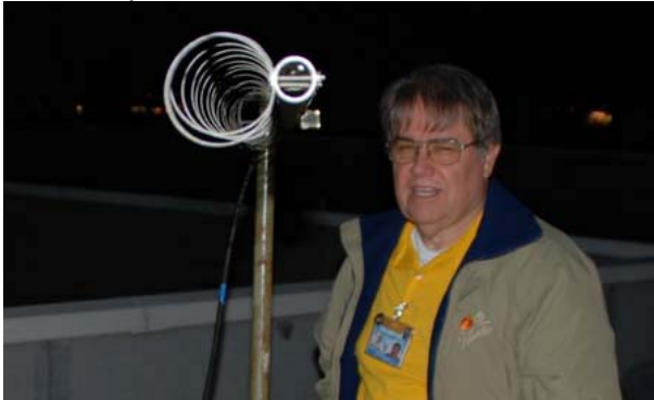
Figure 7 – Robbie KB6CJZ set up a 24-ele Loop-Yagi on the OPD roof and received perfect DATV pictures
