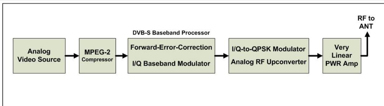
Figure 2 – Block Diagram of DVB-S Transmitter for Digital-ATV
