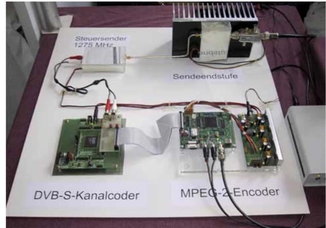
**Fig 4 – Prototype DVB-S D-ATV transmitter like Fig 2**
