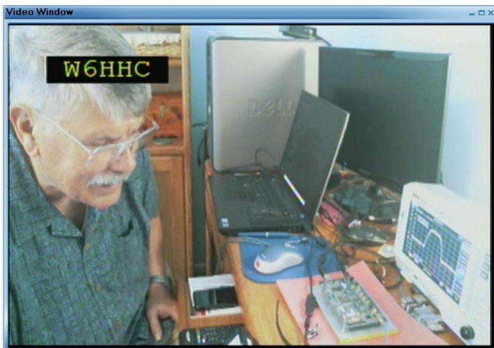
Figure 06 – The VIDEO IDENT feature can be enabled to display your call letters on the received transmission
