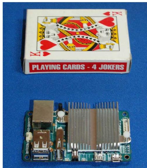
Figure 3 - Size of quadcore-ARM ODROID-U3 board is about the same size as Raspberry Pi
