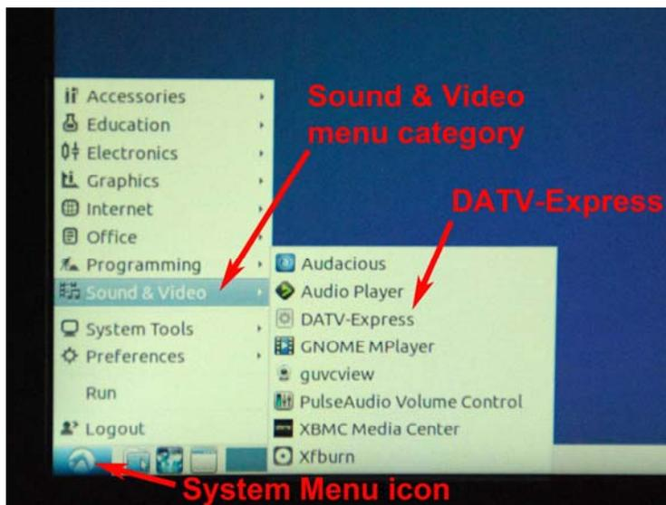
**Figure 6 – The DATV-Express application can be launched from the System Menu of the Ubuntu Desktop**
