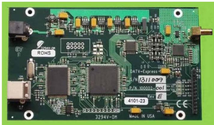
Figure 1 – Production DATV-Express hardware board for Digital-ATV
