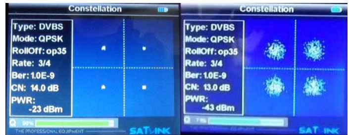
Fig 05 - On the left is the clean QPSK modulation Constellation from new second board etch layout. On the right is the noisy QPSK Constellation from the original board etch layout.
