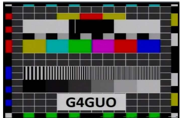
Fig 10 – Test pattern received using DVB-T protocol with 7 MHz bandwidth on 1.3 GHz
